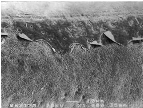
Figure 5 The peeling off of the surface of the activated carbon hollow fiber ( \times 1000 ).
